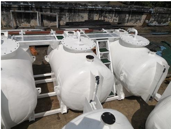
Chemical Storage Tanks with Platform
