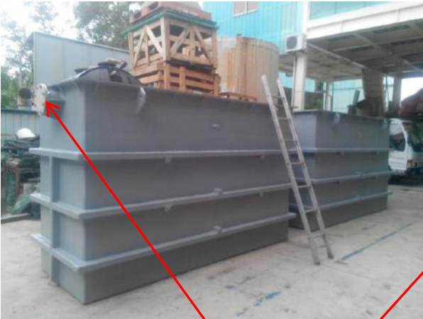
FRP flange inlet
