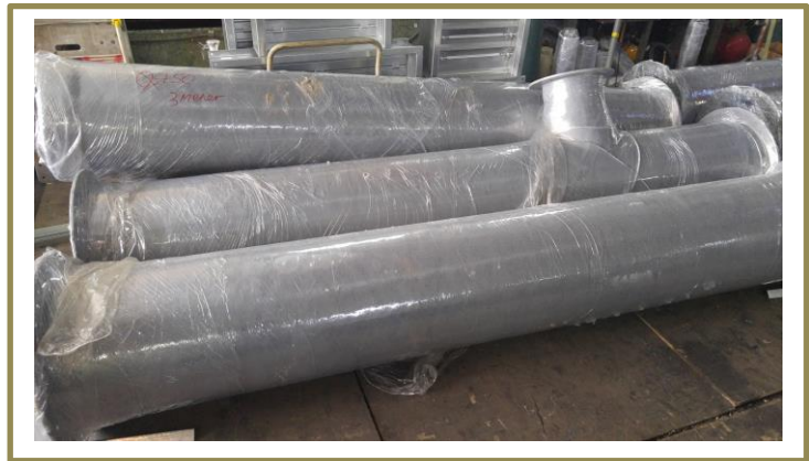
Round ducts and fittings of various sizes for an additive production plant in Jurong Island
