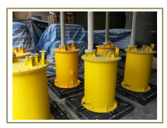
Chemical storage tanks undergoing hydrostatic test
